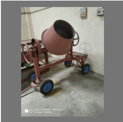
Half Bag Concrete Mixture
